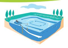
**HYDROPULSE** is a hydro-ejector with a vacuum turbine which reconciles the ventilation and the setting in motion of the masses of water.
